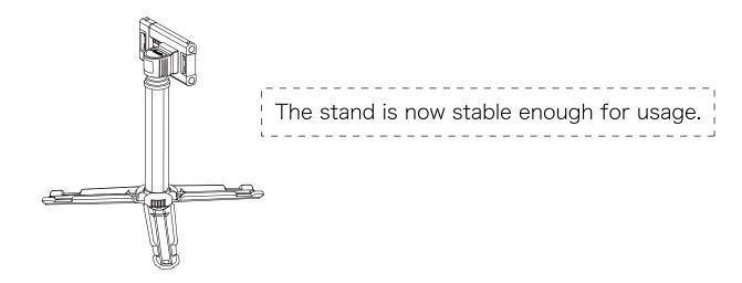
4. Pull out the Central Column and/or Flexi-Arm to adjust height.
