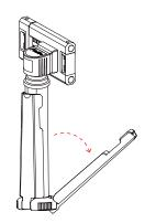
2. Turn the legs while holding the Central Column until all three Openings on the Leg Joints are sealed.
