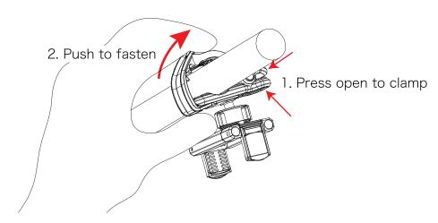
Compatible pole/tube size: (ø17.4 ~ 22mm)
