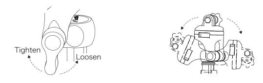
2. After adjustment, tighten the Head Lock to secure.
